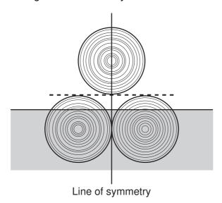
The proportion of the lower logs submerged can be calculated as shown: Taking the volume of one log to be 1 unit, then the amount below the water is 59% of 3 units = (0.59) x 3 units = 1.77 units.
